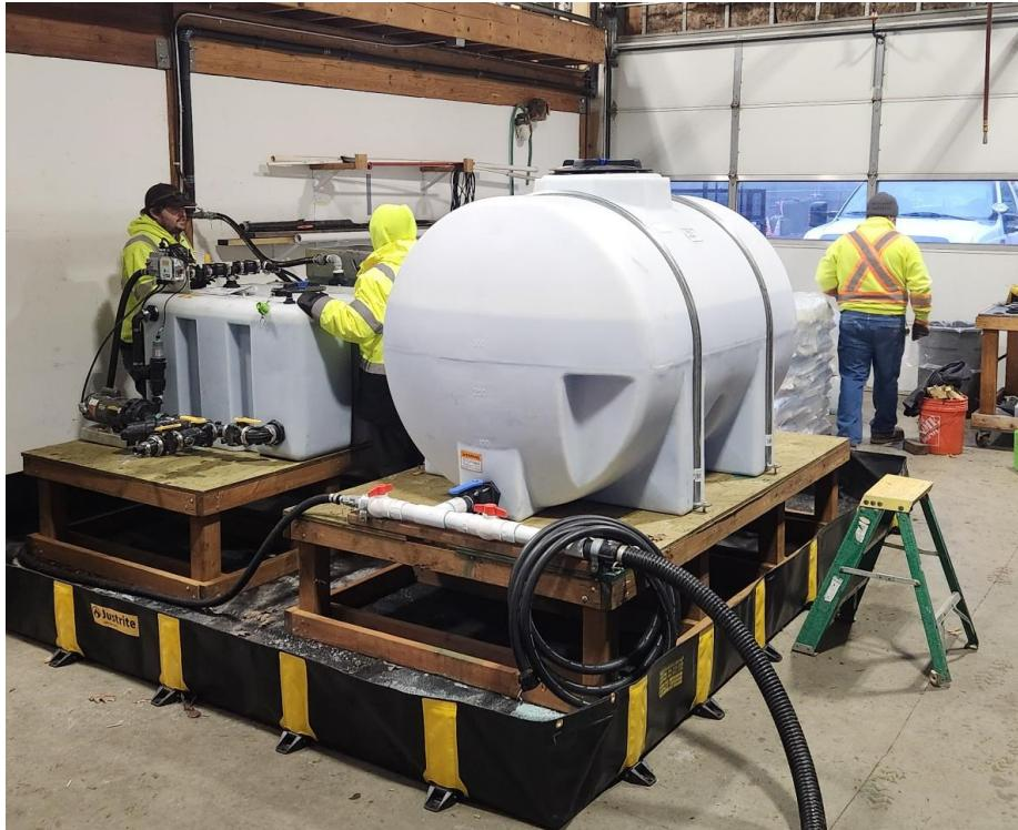
Our brine maker produces brine as needed at a low cost. This improvement saves money and helps to ensure roadway safety during freezing temperatures.
