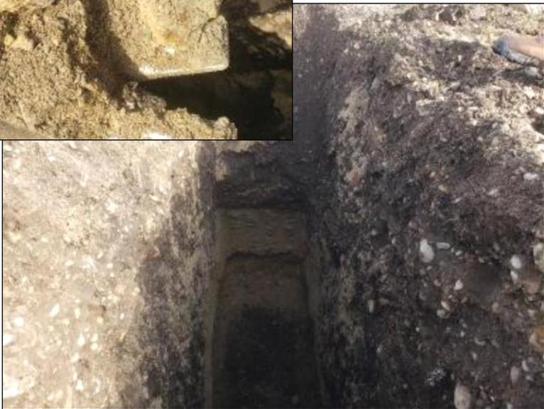
GTP-102 was terminated approximately 8½ feet below ground surface. No groundwater was observed at the time of excavation.
