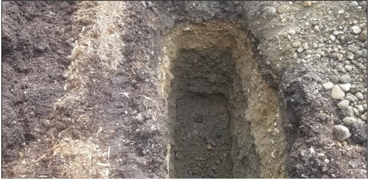
Figure 7. Representative photograph of the subsurface conditions observed in test pit excavations
