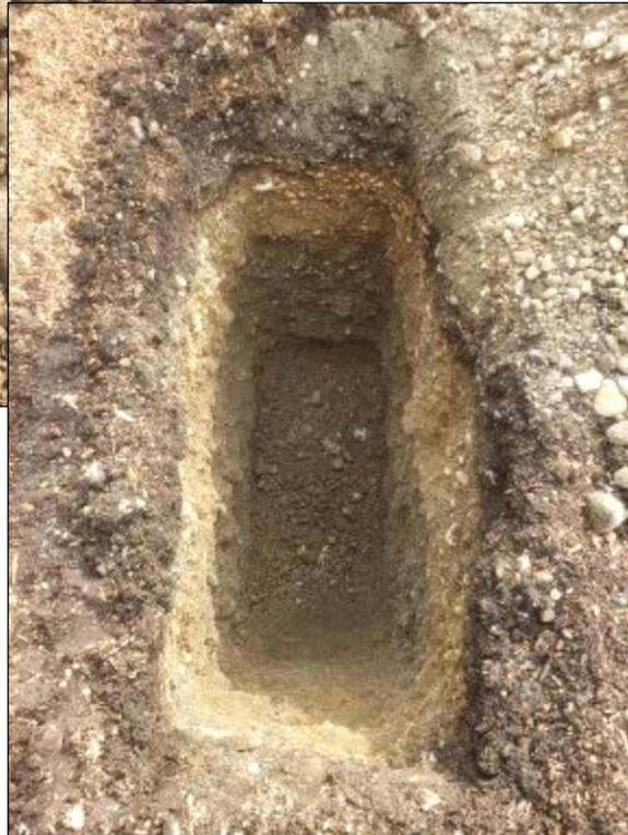
GTP-104 was terminated approximately 7 feet below ground surface. No groundwater was observed at the time of excavation.
