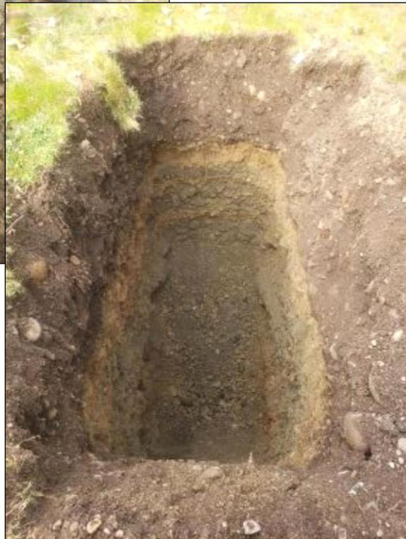
GTP-103 was terminated approximately 7 feet below ground surface. No groundwater was observed at the time of excavation.
