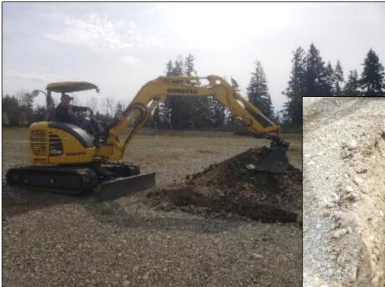
**Photos GTP-106:** Test Pit GTP-106 to approximately 8 feet in depth (below); Operator digging test pit (left)
