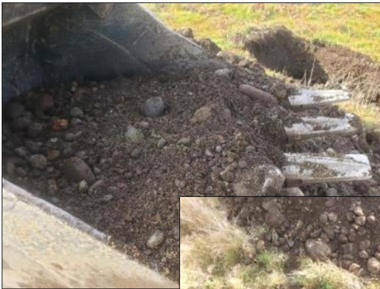
**Photos GTP-101:** Test Pit GTP-101 to approximately 4 feet in depth (below); Sample from bottom of exploration at 4 feet (left)
