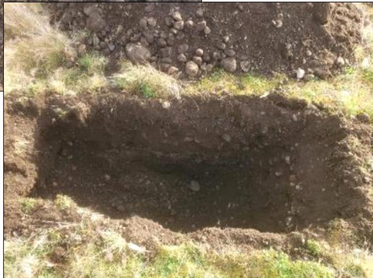
GTP-101 was terminated approximately 4 feet below ground surface. No groundwater was observed at the time of excavation.
