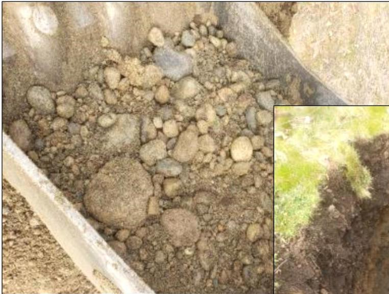
**Photos GTP-103:** Test Pit GTP-103 to approximately 7 feet in depth (below); Sample from bottom of exploration at 7 feet (left)
