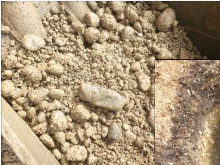
**Photos GTP-104:** Test Pit GTP-104 to approximately 7 feet in depth (below); Sample from bottom of exploration at 7 feet (left)
