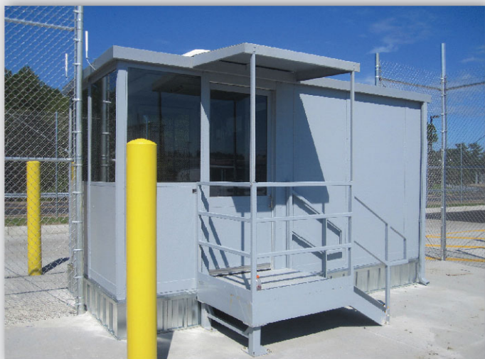
Model 18388 Duraluminum with total exterior paint finish, tinted glazing, factory plumbed integral restroom, canopy over door, raised platform, stair and landing
